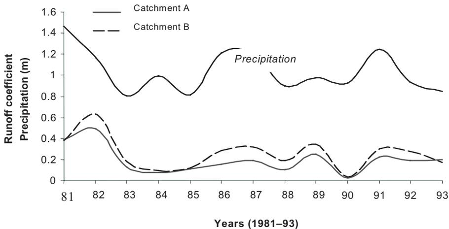
Fig. 3. Runoff coefficients of two experimental watersheds between years 1981 and 1993.
